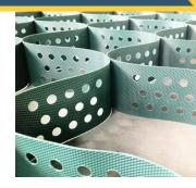
Geocell confines and stabilises the surface of weak soils by creating a honeycomb of interconnected polymer strips that form pockets to locate and strengthen the infill material. Geocell can be laid over stable steep slopes where the cell walls provide a tensile force increasing the strength of the material and acting as mini weirs to reduce run off velocity and soil loss.
